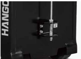
Standard non-detachable tow coupling device, which improves the operation efficiency of the truck.
