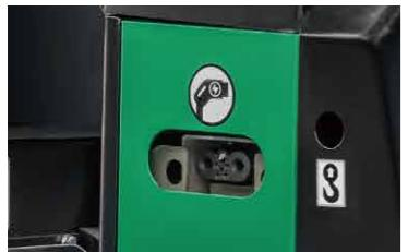
The battery is standard with side charging, which is convenient and fast; the battery can be lifted and removed from the side, making replacement convenient.
